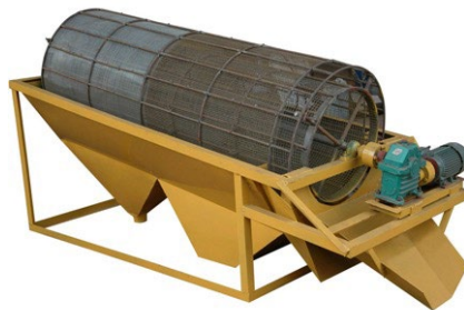
Sorting of the fine fraction at the trommel
