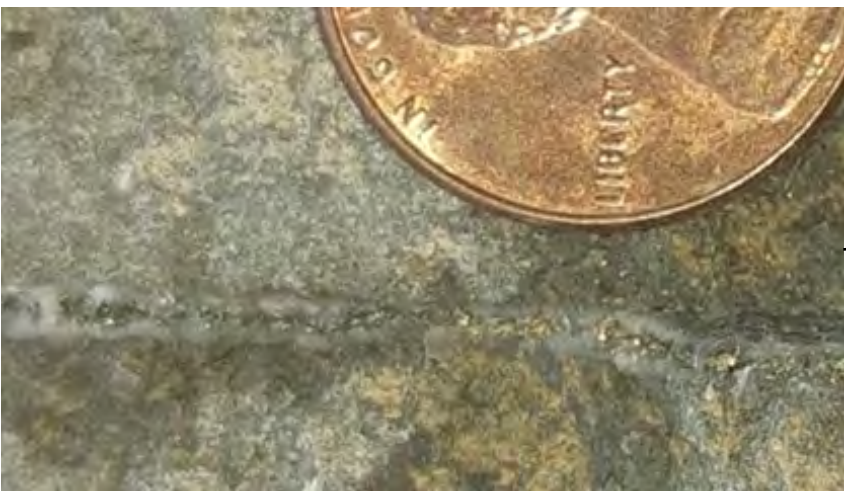
• Example of Quartz vein with central suture of pyrite, chalcopyrite and covellite
