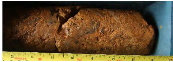
Mineralized fault breccia in hole SH-004 (2.5m @ 9.98% Zn, 4.4g/t Ag)
