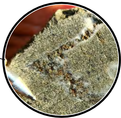
Example of Quartz vein with central median of pyrite and chalcopyrite
